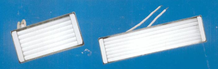
A resistance wire is enclosed in a small diameter quartz tube running parallel to each other and mounted in a special housing. The two sizes are designed to be installed in the same dimensional spacing as the ceramic infrared elements.
